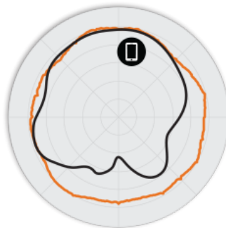
Figure 3. R310 5GHz Azimuth Antenna Patterns
