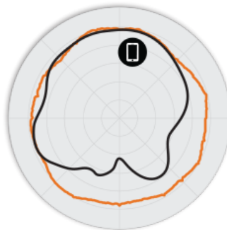
Figure 3. R310 5GHz Azimuth Antenna Patterns
