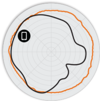
Figure 2. R310 2.4GHz Azimuth Antenna Patterns
