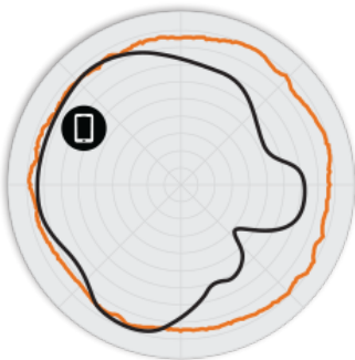
Figure 2. R310 2.4GHz Azimuth Antenna Patterns
