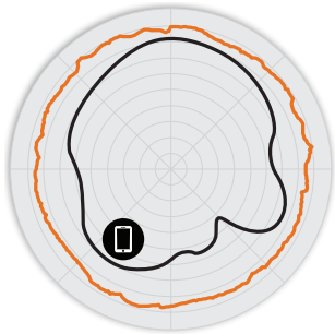
Figure 2. E510 2.4GHz Azimuth Antenna Patterns
