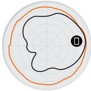
Figure 3. E510 5GHz Azimuth Antenna Patterns
