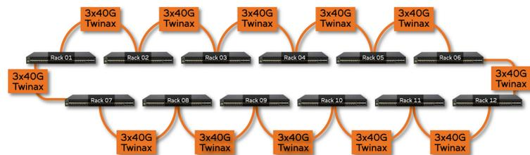
Figure 1: OICR HPC cluster Ruckus network ring.
